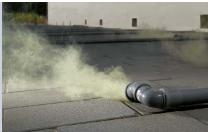
Paving stones with photocatalytic effects reduce the levels of nitrogen oxide and organic hydrocarbon compounds in the air. Source: F.C. Nüdling Betonelemente GmbH & Co. KG
